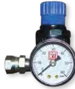
**MR-1** Mini paint gun regulator with up to 30 scfm (850 l/mn), 0-60 PSIG (0-4.08 Bar) operating range for precision adjustment, and features a .25in (6mm) inlet/outlet and chrome glass lens gauge.
