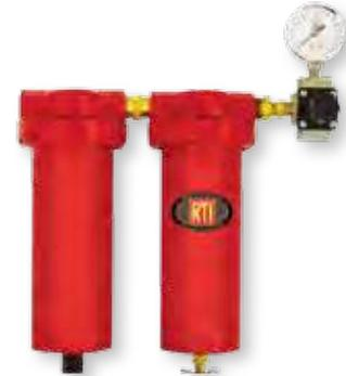
**STEALTH 6060B** .5in (13mm) inlet dual-stage filter system with .375in (10mm) final regulator and first stage auto drain. It uses activated carbon to remove water, dirt, oil, oil vapor and includes two BK-1 mounting brackets.
