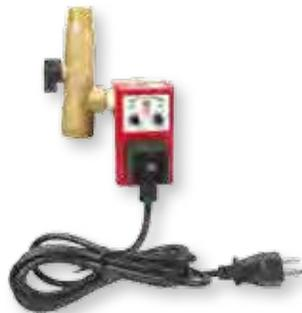
**ED-2-4** Electronic timer drain with indicator lights. Automatically drains water from tank and features a solid brass ball valve with stainless strainer to protect the valve. Manual override comes standard, fits .25in (6mm) or .5in (13mm) NPT.
