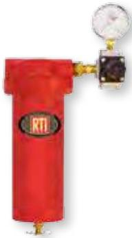
**STEALTH 7000B/7800B** .5in (13mm) inlet. Dirt and oil filter system. Filters to 0.01 micron and comes with .25in (6mm) regulator and gauge. Includes BK-1 mounting bracket. STEALTH 7800B does not include regulator and gauge.
