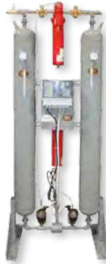
**PERF-180HD** Mainline desiccant drying system that handles flow up to 50 HP compressors, delivers -40° F (-40° C) dew point air throughout shop, and comes complete with 0.01 micron pre and final filter.
